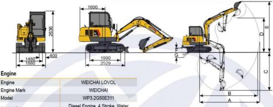
Engine Mark Model Diesel Engine, 4 Stroke, Water **Engine Type** Cooled Number of Cylin-4-98×105mm der-Bore×Stroke Engine Power / Speed 36.8kW / 2200rpm Engine Torque / Speed 200N·m / 1400-1700rpm Displacement 3.17L **Fuel Tank Capacity** 110L
